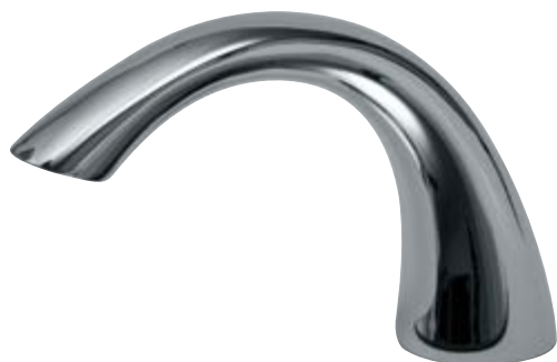
ETAP 3 STAGE 3 odlew po procesie niklowania cast after nickel plating
